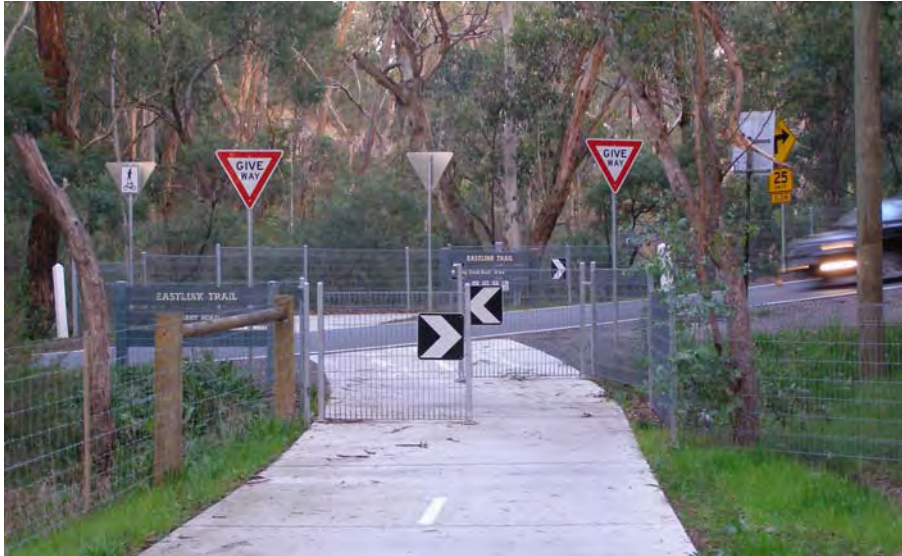
Figure 7.14: Staggered fence treatment
